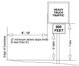
Figure 1: Sign Placement Dimensions
